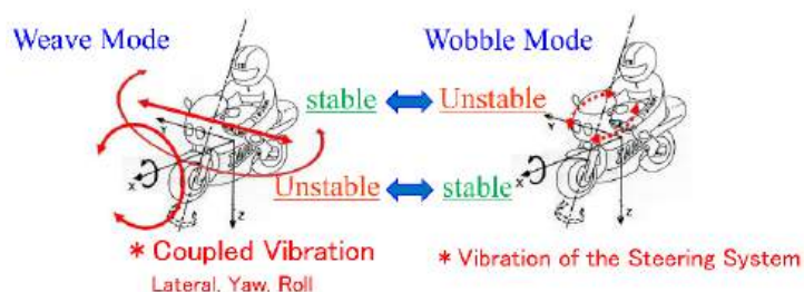
Fig.1 Stabilization Compatibility of Weaved and Wobble Modes
